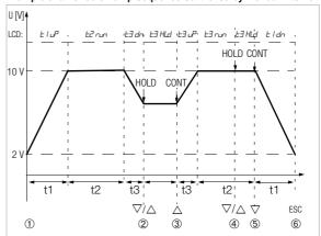
**Ramp parameters:** output quantity: U (range of 0 ... 15 V),  $5 \pm Rr \pm 2$  V, Erd = 10 V, E = 5 s, E = 8 s, E = 5 s, e = 6 Ference for periodic ramps
