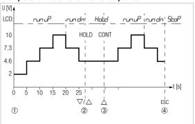
**Interval parameters:** output quantity: U (range of 0 ... 15 V), SER-L = 2 V, End = 10 V, number of interval SEEP5 = 3, L I = 5 s, PadE = Ruba
